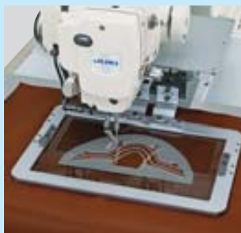
AMS-221EN-HS2516 Shape-tacking of a toe box
