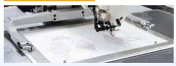
The machine performs various kinds of stitching, making the most out of its wider sewing area in various sewing applications such as attaching handles to bags and pouches, attaching belts, sewing many small parts at a time, attaching parts to shoes and sports shoes (one pair of shoes) and sewing air bags.
