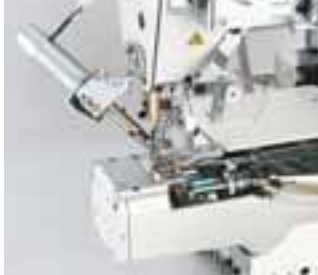
Electromagnetic needle thread / looper thread trimming device
