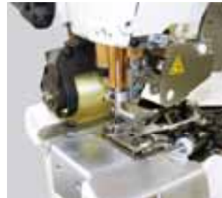
Pneumatic type bottom thread trimming device
