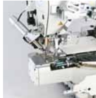
Electromagnetic needle thread / looper thread trimming device
