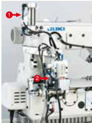
① Presser lifter drive mechanism air cylinder ② Thread trimmer drive mechanism air cylinder
