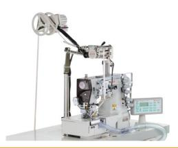
The tension-adjustment type elastic feeder (MU) feeds the elastic lace according to preset data while adjusting tension exerted on the elastic lace, so uniformly finished and quality products are obtained.
