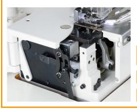
Thanks to the differential feed ratio regulator (AI) , the differential feed ratio can be automatically switched by stitch counting, so this machine sews the fabric uniformly in any direction, wale, course or bias.
