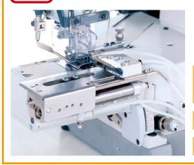
This sliding type hemming guide folds the fabric to form a hem in hemming operations. Thanks to this device, hemming is easy and resulting hem width is uniform, so quality products are obtained. Two types of driving sources are available, pneumatic and electric.
