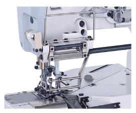
The elastic lace feeder with a mechanical metering device (MD), feeds the elastic lace according to the feeding amount of fabric that is fed, so that the feed of the elastic lace is even if the machine speed is changed. This results in uniform and beautiful elastic lace attaching operations.
