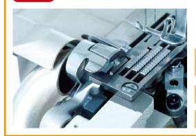
This is a device that trims the edge of the fabric when interlock stitch machines perform hemming, tape attaching or elastic inserting operations. The edge of the fabric is evenly and neatly finished.
