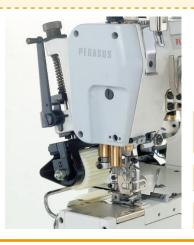
The roller pulls the fabric from behind the needle drop hole. Thanks to this device, the machine smoothly sews difficult-to-feed fabrics, providing beautifully finished products with no plyshifitng.
