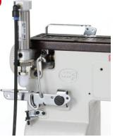
Pressing the treadle with your heel raises the presser foot. This device is easy to use, thus decreasing operator fatigue and increasing productivity.
