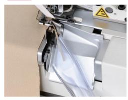
This pneumatic device strongly sucks up cutting waste and fine dust generated during sewing, providing clean and comfortable working conditions.
