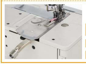
The suction inlet is positioned flush with the needle plate and right behind the presser foot. Thanks to this feature, wide, double chainstitch, extra heavy weight or woolen thread chains are smoothly sucked up.
