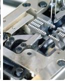
If the looper thread is pulled at the end of sewing, this thread trimmer prevents unraveling with STITCHLOCK. Use of this thread trimmer eliminates the need for a bartacker. In addition, there is no need to perform manual thread trimming using scissors. As a result, the quality of sewn products and operational efficiency is dramatically increased.
