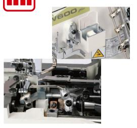
This device reliably reduces heat generated at the point of the needle by friction when they penetrate the fabric with the machine running at high speed. In addition, it allows the thread to move smoothly through the machine, decreasing the cause of stitch skipping and/or thread breakage. As a result, the machine produces uniform stitches.
